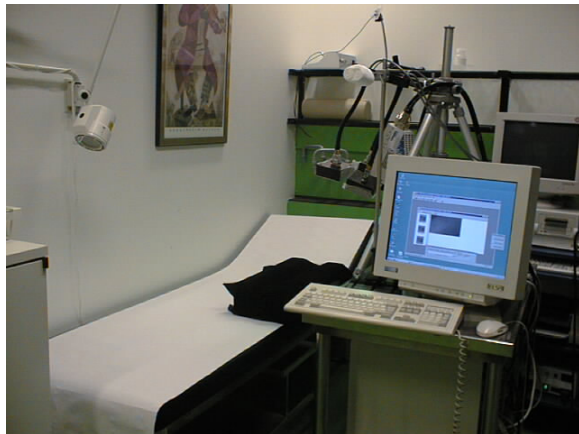
Fig. 10. PPGI setup for measurement of a subject in supine position [10].
